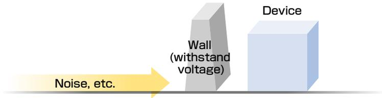
Abnormal voltage higher than the withstand voltage
