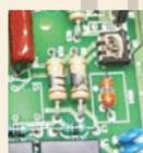
Integrated circuit and resistor damaged by lightning surge
