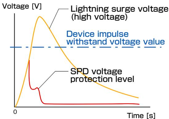
Voltage no higher than the withstand voltage
